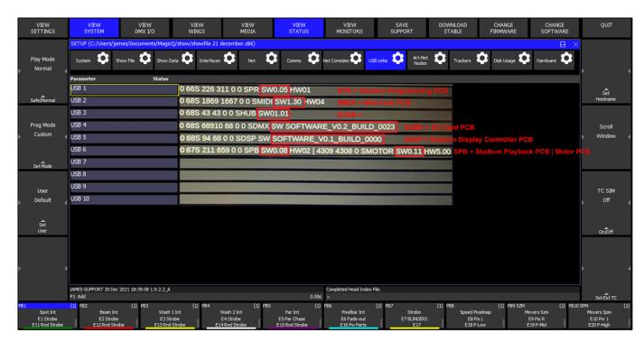
To check the version of firmware in use go to Setup, View System, View Status and select the Hardware tab. For each panel/board it shows current version, available highest firmware version and current update status.
