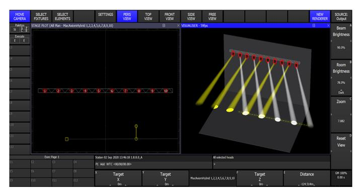
The *Base Position* is the starting position for the heads before they are panned around to focus on the point. If the head has to pan more than 90° from the base position then it will *flip* the head over. The default base position is directly downstage. If the lights flip while they are moving between positions then a different base position may be required.
