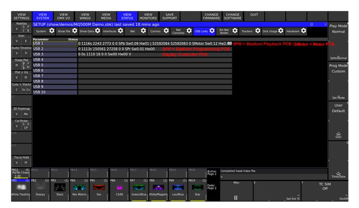
To check the version of firmware in use go to Setup, View System, View Status and select the Hardware tab. For each panel/board it shows current version, available highest firmware version and current update status.
