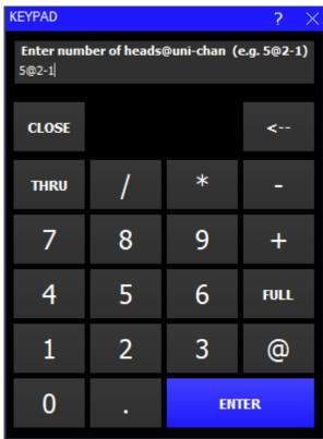
To patch a head at a specific address use @. For example to patch 10 dimmers at DMX address 20 key in 10@20. To patch to the
