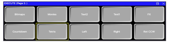
Buttons can also be set as solo buttons (also known as radio buttons) so that a group of buttons programmed as Cues or Cue Stacks can be set so that only one of the group is active at a time. Use soft button E to select "Solo".
