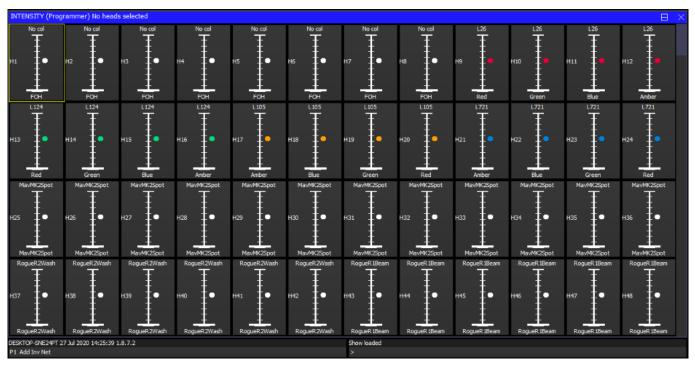
The SQUARE OFF soft button enables fast programming of intensities. Using the touch screen select the channels you wish to have at full and at zero – but don't bother being exactly accurate with the level of the selection. Pressing SQUARE OFF finishes the job by setting all channels that are less than 50% to 0 whilst setting channels above 50% to full.
