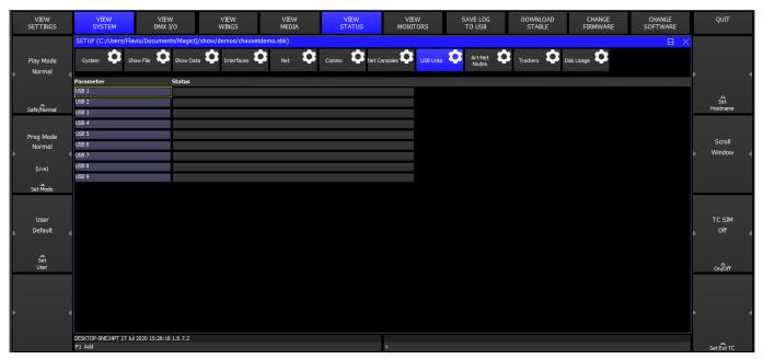
Put the cursor on the line for USB 1 as above. Press CHANGE FIRMWARE and select the new firmware file - e.g. CH331\_V1.0.hex.
