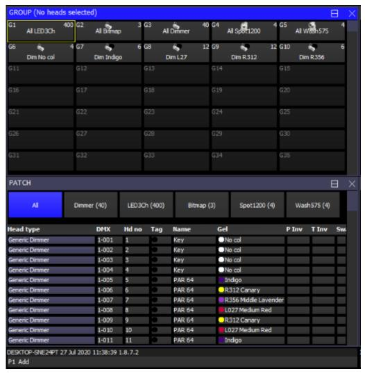
A window is displayed by pressing the appropriate window button. On MagicQ PC/Mac the window can be selected from the Window Menu from the toolbar. Changing window does not affect programming or playback.
