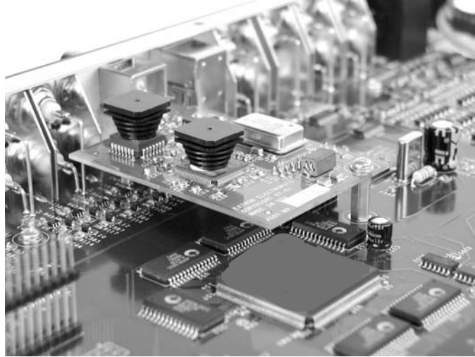
Installed SDI input card
