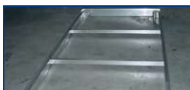
2 Traverses de renfort 2 reinforcement griders
