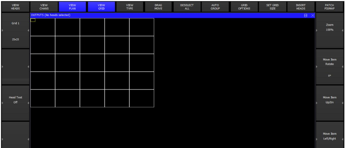
Note that it is not necessary to allocate a head number to every position in the grid – so if your LED heads are placed at weird angles you can make a grid with the LED placed as you would see it. Multiple grids can contain the same head numbers – so it is possible to have one grid with the LED tightly packed and another representing how they are really spaced out.
