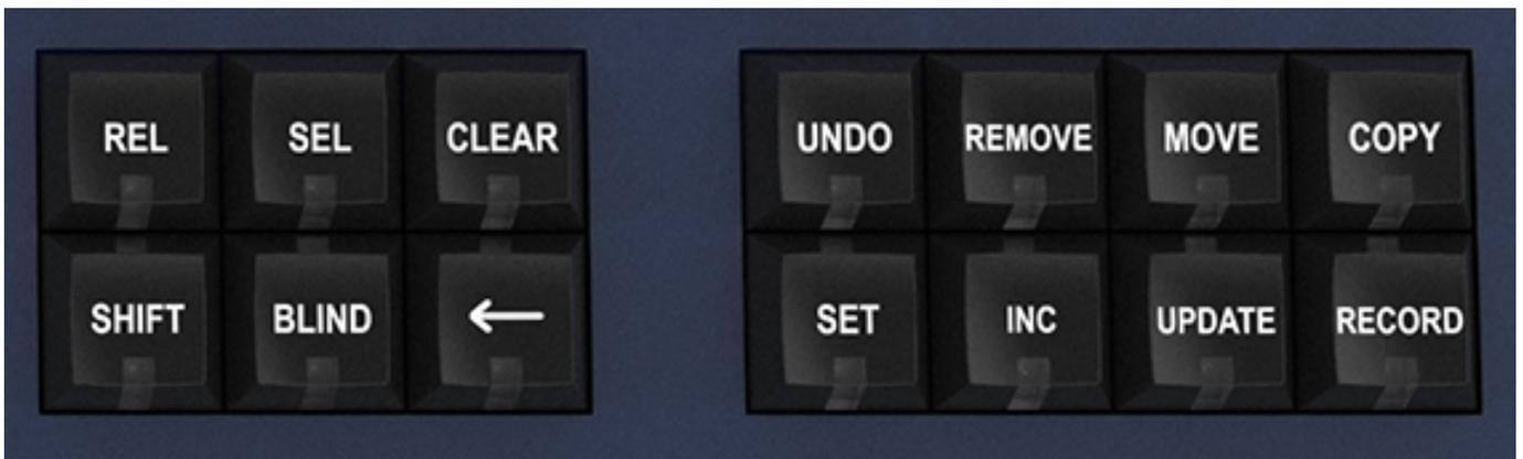
The Editor buttons are used to modify program data. The 8 buttons on the right hand side are the action buttons which are used to modify show data. The action buttons are UNDO, REMOVE, MOVE, COPY, SET, INCLUDE, UPDATE, and RECORD.
