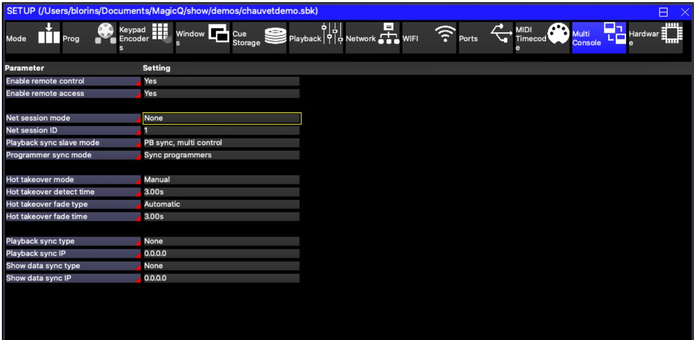
Configure the master console by setting the multi console setting "Show data sync type" to "Master Prog".
