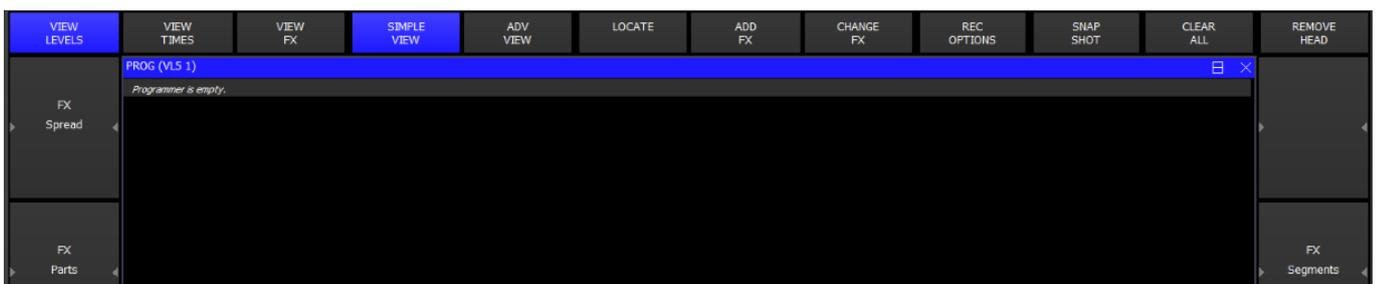
In the Channel Times and Channel View windows you have a choice of a Simple View or an Advanced View. The Simple View is sufficient for most programming – it enables modifications of fade times on a per attribute type basis and modifications of each programmed FX. The Advanced View enables fade times and FX parameters to be set up on a per channel basis.
