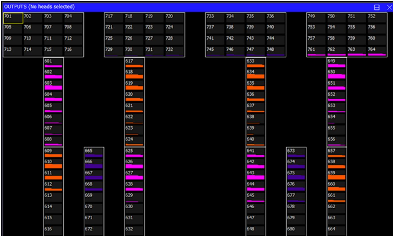
In the Outputs Window, select View Plan. Then select View Grid and View Hd Nos. Press Grid Size and enter a matrix size for your lighting rig – e.g. 30/20 gives a 30 column by 20 row grid.
