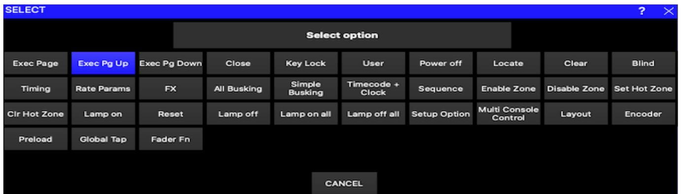
There are special functions for controlling universe zones – enabling, disabling and setting the hot takeover state. These enable complete control of complex DMX routing from a simple interface.
