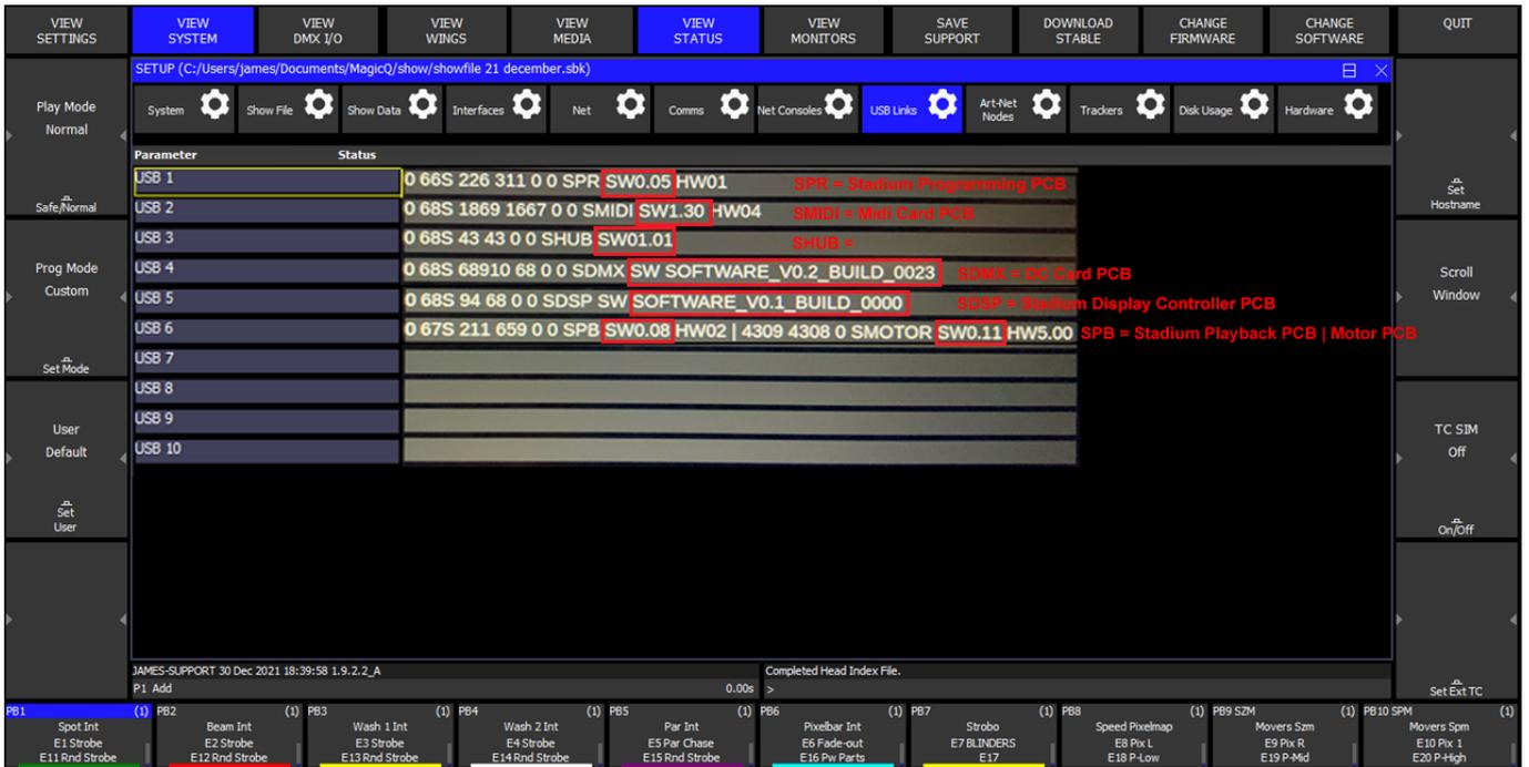
To check the version of firmware in use go to Setup, View System, View Status and select the Hardware tab. For each panel/board it shows current version, available highest firmware version and current update status.
