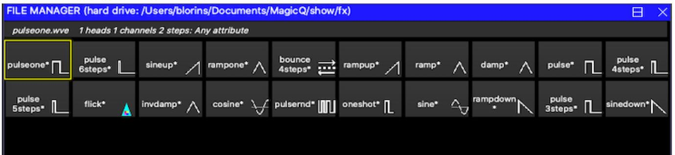
You can apply multiple FX to a head, provided that the FX uses different attributes - e.g. you can mix a Pan Sine with a Tilt Sine. Once you have chosen a FX you are returned to the Prog Window. Use the encoders to modify the parameters of the FX such as the speed, size and spread between heads. By default FX size goes up to 255. Hold SHIFT and use the encoder to get sizes above 255.
