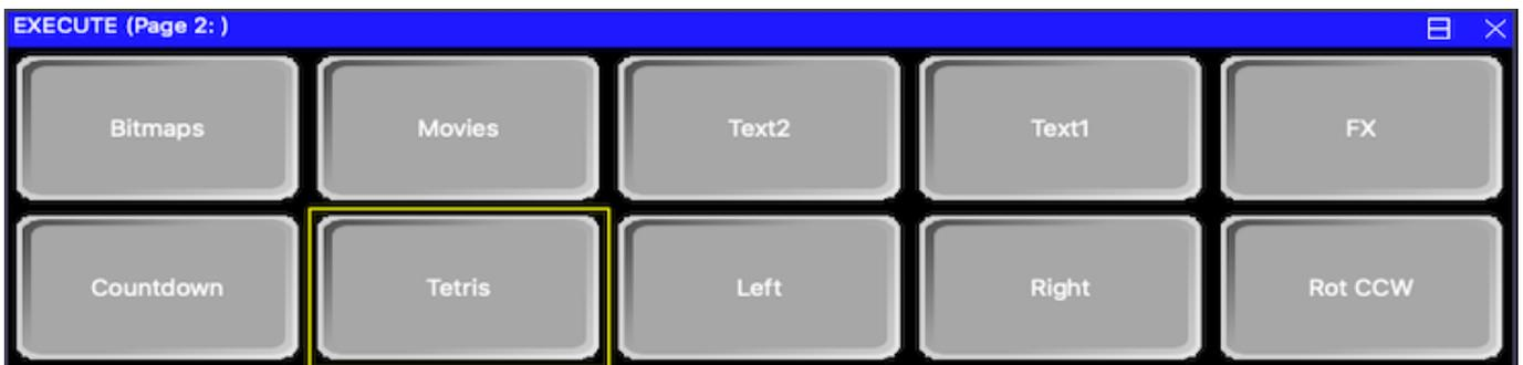
Buttons can also be set as solo buttons (also known as radio buttons) so that a group of buttons programmed as Cues or Cue Stacks can be set so that only one of the group is active at a time. Use soft button E to select "Solo".
