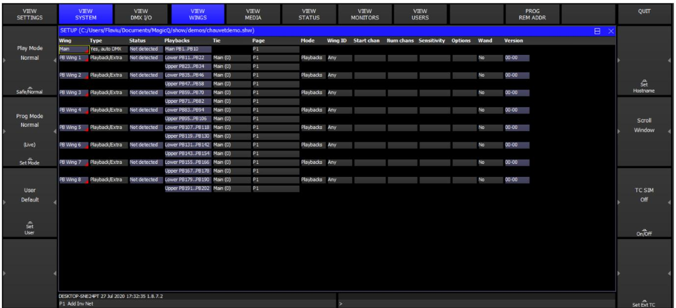
To enable the Scene Setter in MagicQ software, set one of the Wings in Setup, View System, View Wings to "Remote Panels". A "D" in the Status Window shows that the panel is detected. It will then control four Playbacks on that Wing. Playbacks can be programmed on MagicQ from the Playback Window.
