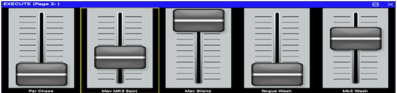
From version 1.8.8.0 MagicQ supports full sizing of all Execute items using the Item Width and Item Height soft buttons and encoders. In previous versions, and in 1.8.8.0 if faders are set to width and height of 1 then the size faders then if there is an unused box below the fader item then MagicQ automatically adjusts in the Execute View to fill the two boxes.
