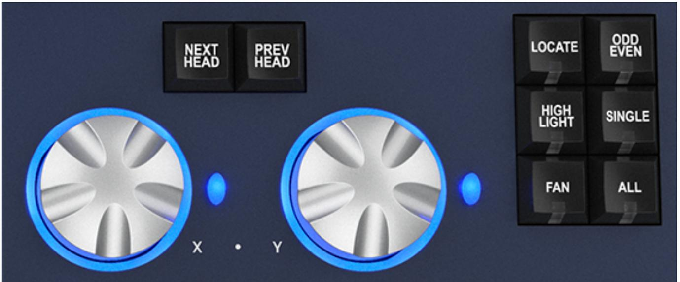
The NEXT HEAD and PREV HEAD buttons are used to select an individual head to modify.
